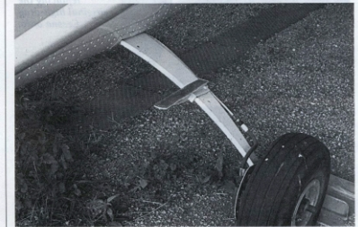
Scaled-down new step on the gear leg (top) cuts drag, but actually serves the human foot quite adequately. Gear legs themselves receive new lower-drag fairings. Lower photo shows the original gear leg and its larger step.
