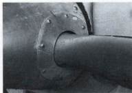
Special cuffs seal the gaps around the spinner's prop opening. The hairy matrix at the spinner/cowling juncture is not a giant bird nest, but an AstroTurf liner.
